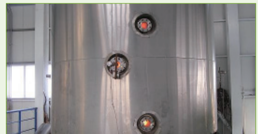
A 24 set energy-saving polycrystalline silicon reductive furnace
